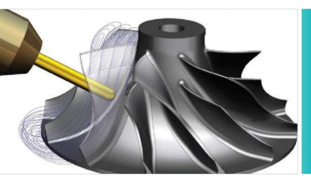
NX Turbomachinery Milling for easy programming of multi-bladed parts
