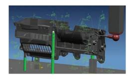
Two approaches enable you to evaluate how much rework will be needed to improve quality of the produced parts – optional analysis modes and the ability to "float" measure data when fitting it to the nominal CAD model.
