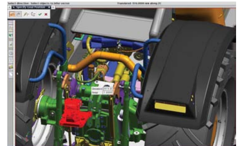
NX assembly validation tools include extraction path planning capabilities that optimize designs so that a product can be easily assembled, disassembled and maintained.
