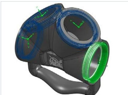
Duplicate assembly components can carry properties unique to each individual occurrence, which is especially useful when using the same component many times in the same product. And these properties can be used in associated drawings.
