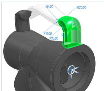
The ability to remove material along a path is now accomplished by sweeping a solid body, simulating a milling operation.
