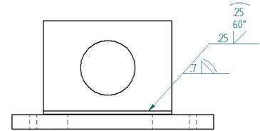
**Stitch weld** Where strength or gas tightness is not a priority, stitch welds are used to save time and materials. The Stitch Weld command provides a dedicated tool to apply stitch welds to join components. Options allow you to control the stitch length, gap size, style and offset values for perfect control.
