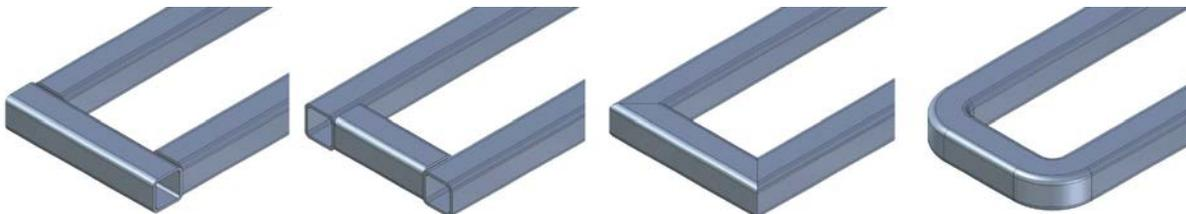
member will have material removed to suit). A butt2 condition is the opposite, with the shortest member being trimmed against. You can mix and match frame component sizes and shapes and their end condition treatments; any combination is possible.
