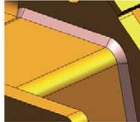
**Customized welds** Not all welds are simply triangular in shape; some beads need to represent a specific cross-section, either because of the weld specification or preparation type. Assembly feature tools – protrusion, revolved and sweep protrusions – are available so that users can define their required weld bead cross-section.
